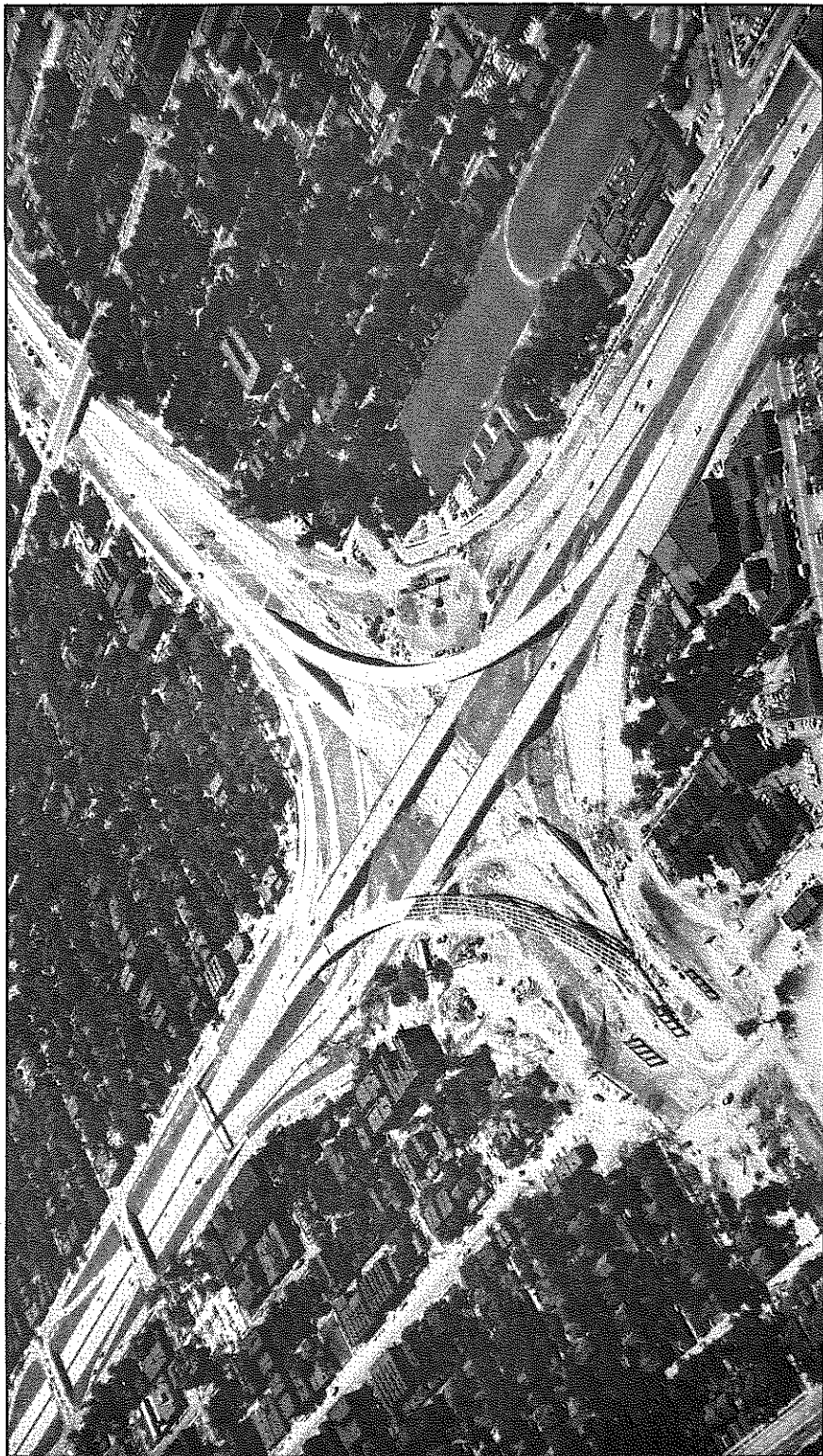
Interchange of the Edsel Ford and John C. Lodge expressways. Looking southwesterly, the Ford Expressway is in the upper right and the Lodge Expressway in the upper left of the picture. When completed, there will be 14 structures making up the interchange which will provide unrestricted traffic flow in any direction.
